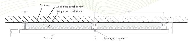
lenofon wood panels and soundproofing materials are combined to form a structure of thickness 90 mm.
