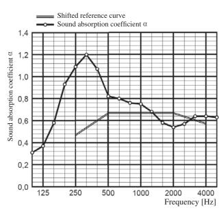
$<sup>\</sup>alpha$ . Sound absorption coefficient according to ISO 354
