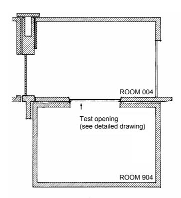
Test rooms. Vertical section. Scale 1:125.
