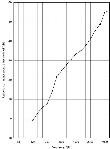
Weighted reduction of impact sound pressure level according to EN ISO 717-2:1997:
