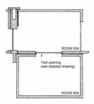
Test rooms. Vertical section. Scale 1:125.
