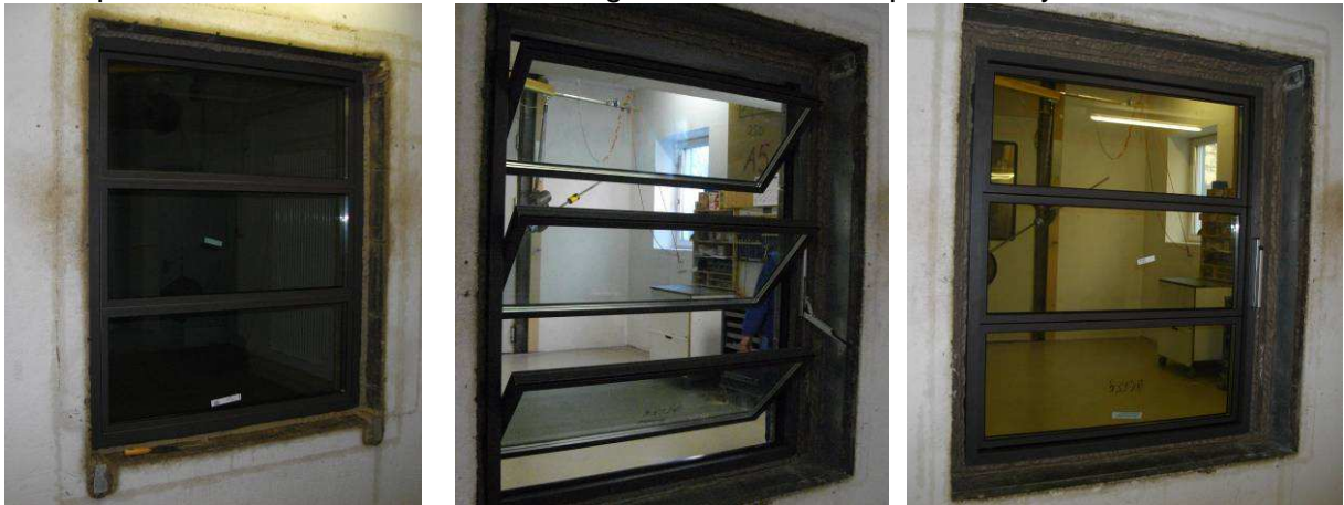
Fig. 1 Photos of the mounted element, created by ift Laboratory for Building Acoustics
