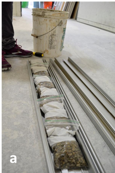
FIGURE 4-12: CLASS B FILLED MULLION (A) PEA GRAVEL (B) SAND (C) MINERAL WOOL (D) MLV PILLOWS
