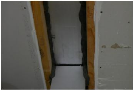
FIGURE 2-12: TEST SPECIMEN OF AN OVERCLAD MULLION ELEMENT AND LOCATION IN THE FILLER WALL APERTURE (IMAGES: © ENCLOS CORP)
