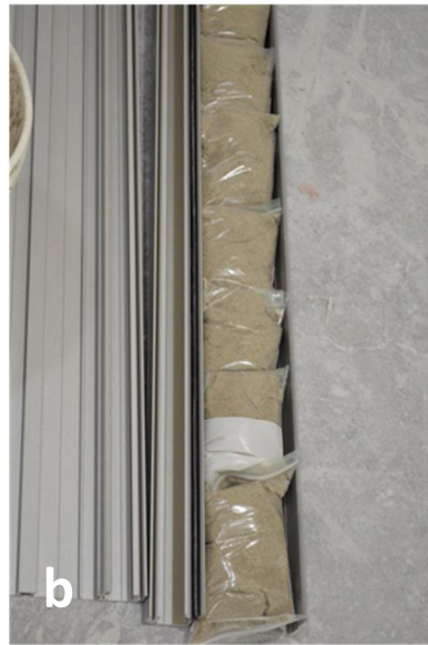
FIGURE 4-12: CLASS B FILLED MULLION (A) PEA GRAVEL (B) SAND (C) MINERAL WOOL (D) MLV PILLOWS
