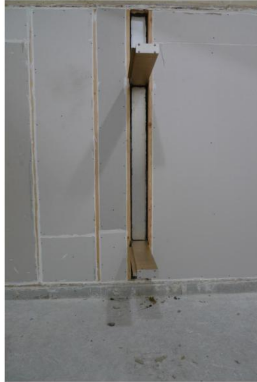
FIGURE 2-12: TEST SPECIMEN OF AN OVERCLAD MULLION ELEMENT AND LOCATION IN THE FILLER WALL APERTURE (IMAGES: © ENCLOS CORP)
