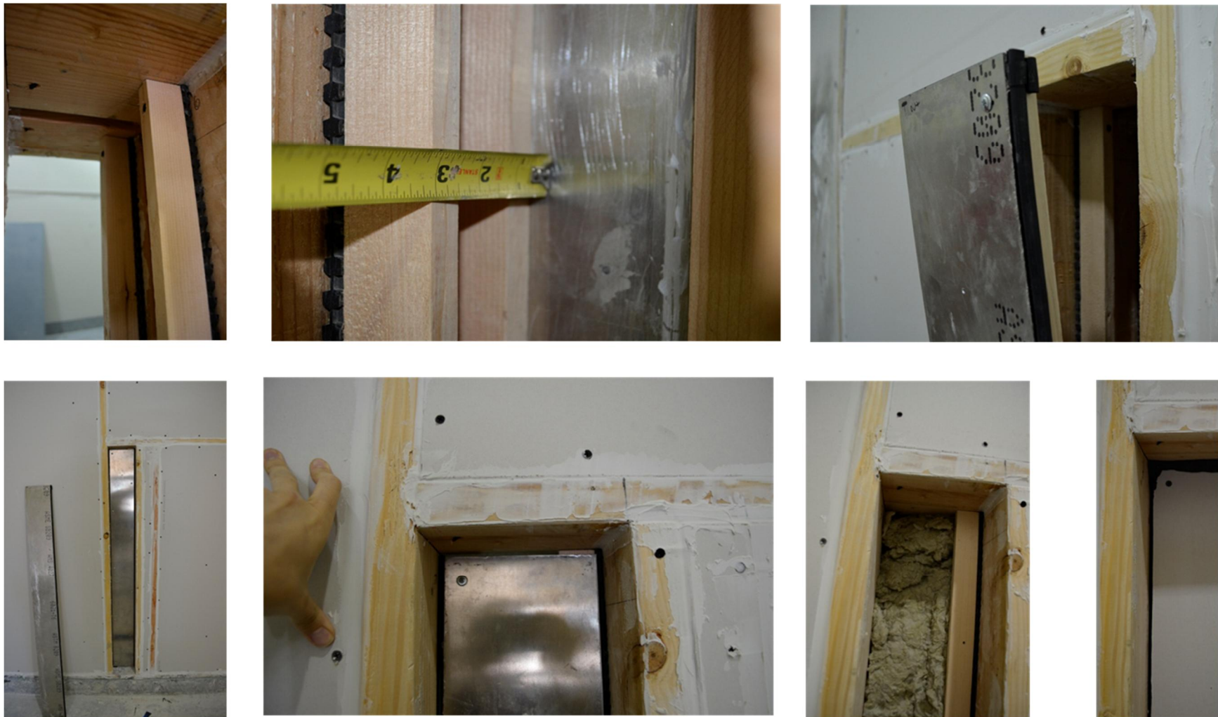
FIGURE 4-48: PHASE 2B CLASS A SPECIMEN CONSTRUCTION OF SOLID PLATE TESTS
