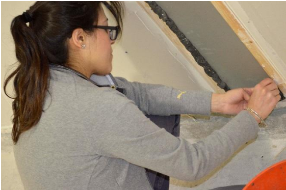
FIGURE 4-6: PUTTY APPLIED TO SPECIMEN PERIMETER EDGE TO SEAL ACOUSTIC LEAKS
