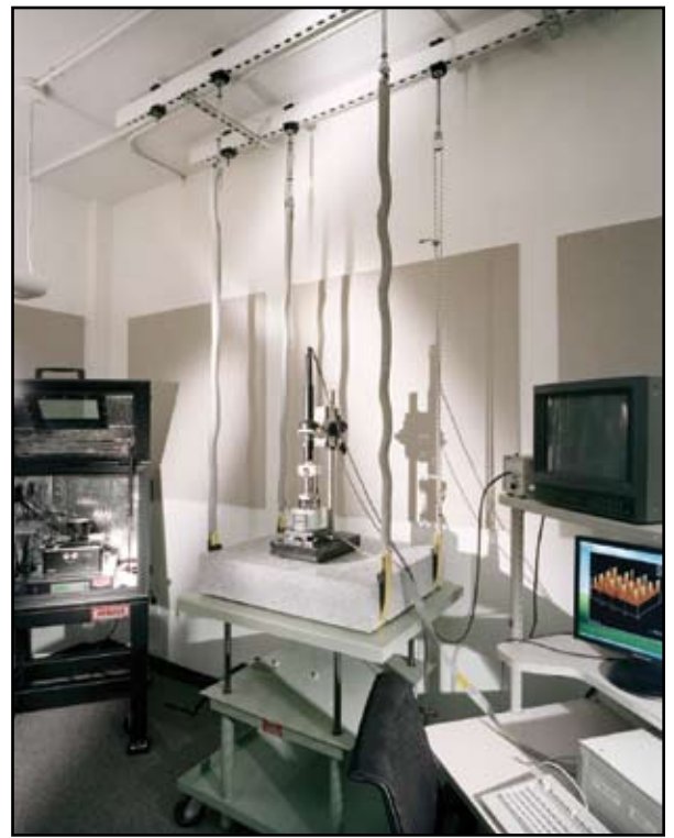
Inertia base suspended with elastic straps; New York University.
