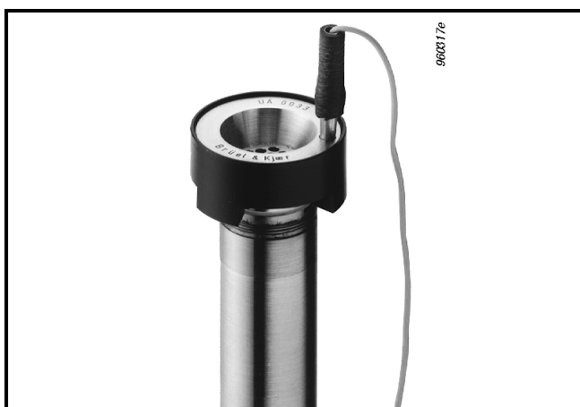
Fig.2.35 Electrostatic actuator used with a 1/2" microphone
