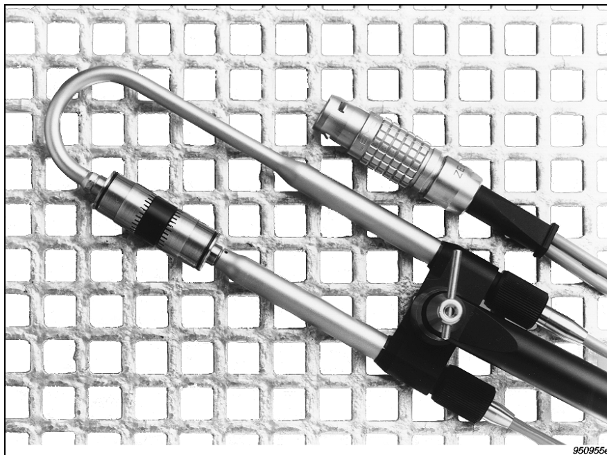
Fig.1.3 Sound Intensity probe using a phase-matched pair of microphones
