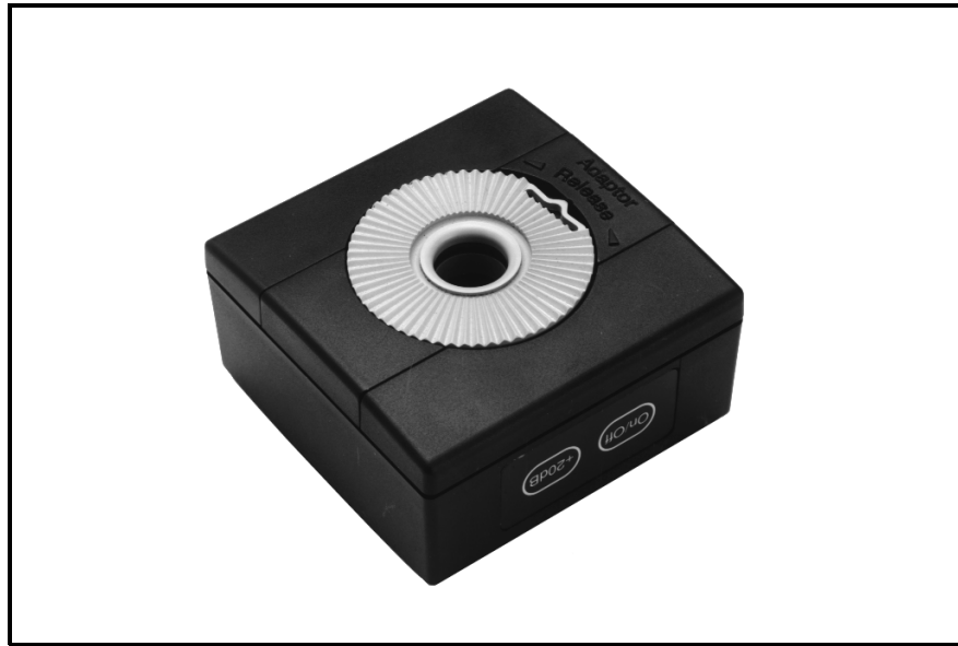
Fig.6.1 Sound Level Calibrator used for field calibration of measurement microphones
