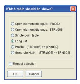
A new feature is included here: now, a profile between sound source and reception point can be indicated. If the source is a line source, you will be prompted to identify the line section whose center is to be the starting point of the profile.
