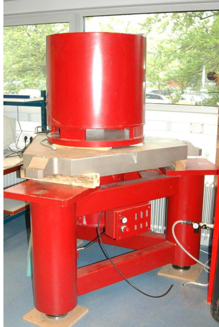
Figure 1.2: Model of a lens and its supporting frame used in a wafer stepper, provided by Integrated Dynamics Engineering GmbH (photo taken at the Mechanical Automation Laboratory, University of Twente)
