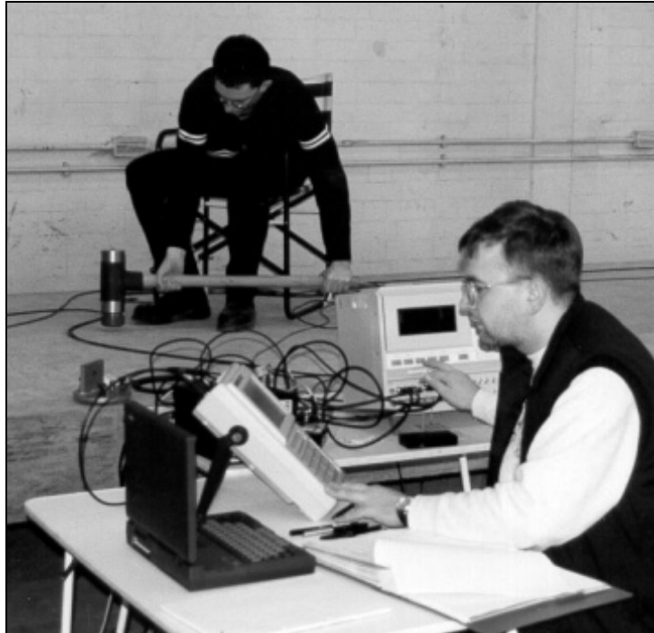
Figure C.2 Typical instrumented hammer setup using a dual-channel signal analyser
