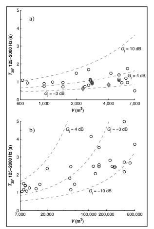
Figure 2: Calculated reverberation time  $(T_{30})$  as a function of volume (V) of a) small and b) large venues.
