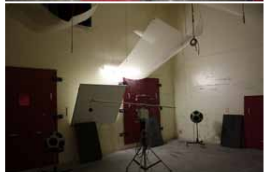
Figure 6.4 Insulation measurements rooms in the Peutz Laboratory. Hanging and standing baffles for creating a practical achievable diffuse sound field. An automatically rotating microphone is installed for accuracy.
