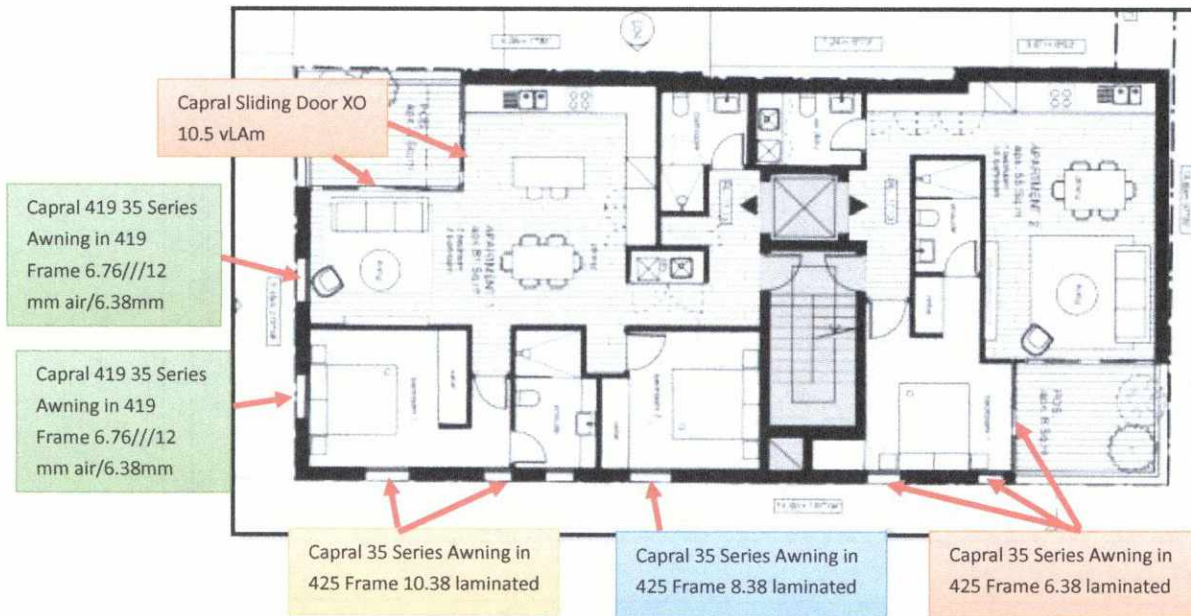
Figure 10 Glazing/Sliding Doors For Level 2
