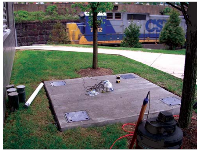
Figure 6. Subscale vibration isolation test floor.
