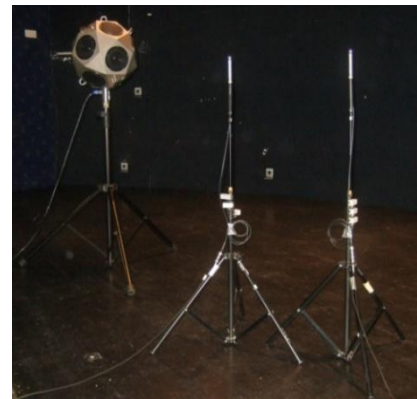
Figure 9: Equipment; laptop and amplifier (left), omnidirectional sound source and two microphones (right)
