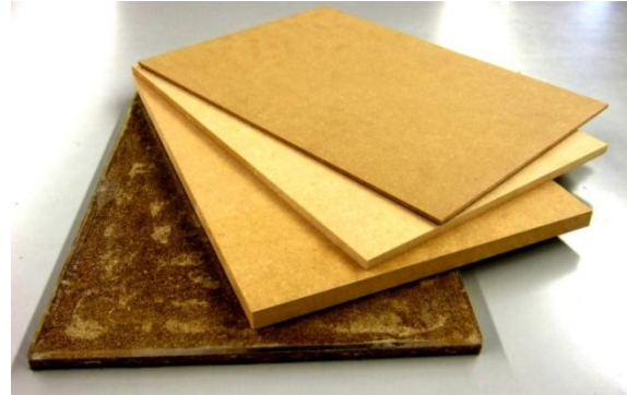
Figure 58: Test specimen, left: MDF 16 mm, XPS sawn side, XPS smooth side (bottom to top), right: Perspex, MDF 16, 9 and 4 mm
