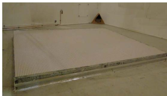
**COEFFICIENT D'ABSORPTION ACOUSTIQUE  $\alpha_s$
