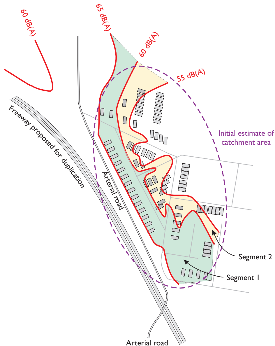
Figure PNIV(c)-7. Example 4: Site layout, L_{Aeq(15hr)} noise contours before noise barrier or architectural treatment, and the noise catchment and its segments (shaded areas).
