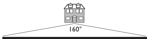
Figure 4.3 A 160° subtended angle at a reception point is generally considered to provide a minimum barrier length. If this barrier attenuated noise by 11 dB(A), an “infinite” barrier (180°) would provide an attenuation of about 16 dB(A).
