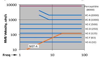
Two new curves called VC-F (63µin/s) and VC-G (32µin/s) were adopted in 2007. In addition, the NIST-A criterion, along with a modified version called NIST-A1, is being used in national labs and university facilities. Our opinion is that VC-F and VC-G are more appropriate to non-floating slab construction such as ground/basement level slabs.
